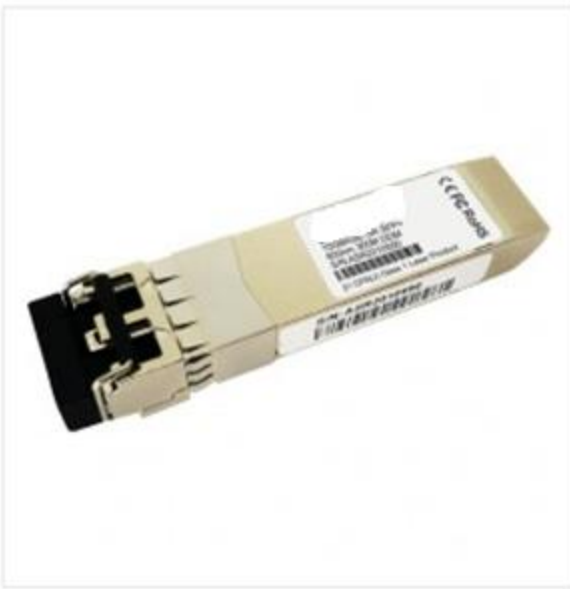
10GBASE-SR SFP+ transceiver module for MMF, 850-nm wavelength, 300m, LC duplex connector
